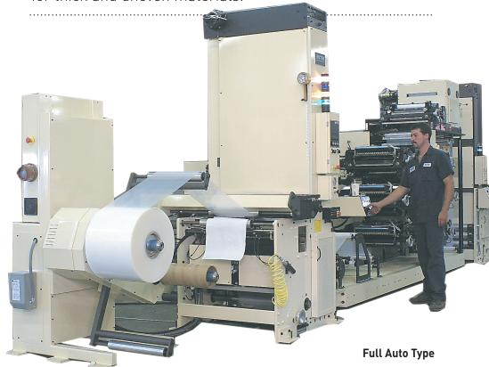
Unlike modular press designs that require long web pass and produce considerable waste upon starts and stops, KPG's design uses a short pass around the CID, ensuring the least waste in handling expensive tube materials and achieving perfect print register with ease. The ultraviolet (UV) curing system cures printing inks instantaneously to ensure clean product conditions.
